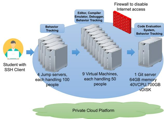
Fig. 2. Integrated environment structure of OS experiments.
